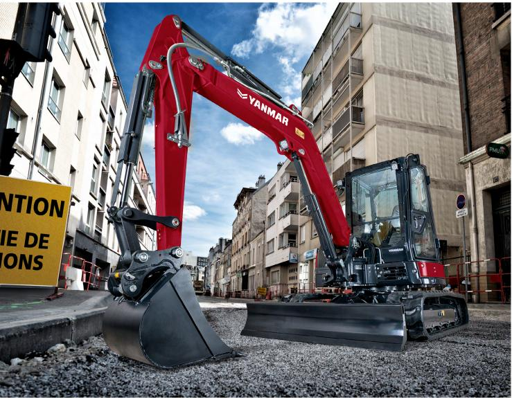
The ViO57-6B benefits from an improved powerline: the combination of the new more powerful engine new Stage V powerful engine with Diesel Particulate Filter, the hydraulic pumps (+ 14 %) and a new control valve improve the cycle-times by more than 10 %.
